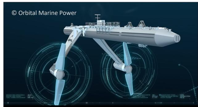
Animation of Orbital Marine Power's 2MW O2 tidal turbine
