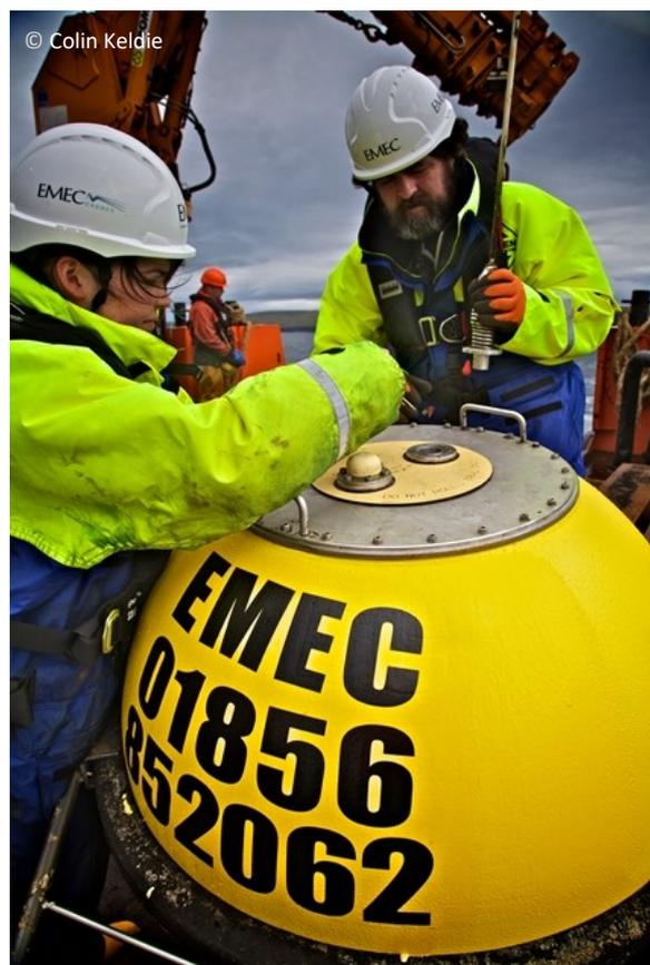
Photo: EMEC operations preparing waverider buoy for deployment.
